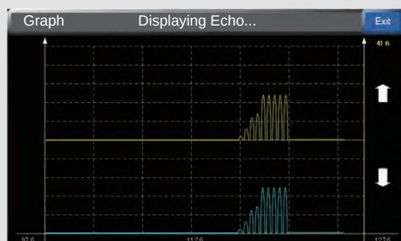
Graph Display of Echo Received Displays ultrasound signal strength. Useful during setup and checking operation.
