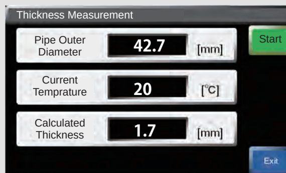
Measures Pipe Thickness Useful when pipe inner diameter is unknown.
